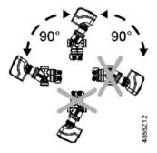
Thermal actuators STA.., STP. , may be installed in any position. Actuators SSA.., SUE.. must be installed horizontally up to 90° and not hanging.
