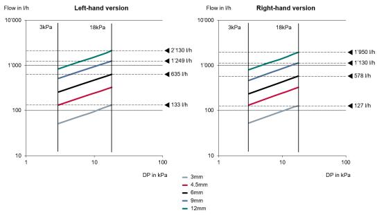
The sizing of the orifice plate and the PICV should be based on the required flow range of the Valve Kit. An orifice plate that is too large results in a lower measuring accuracy. An orifice plate that is too small causes a high pressure drops and leads to increased energy consumption.
