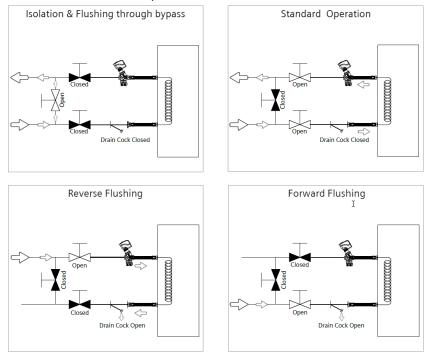
Isolation & flushing through bypass: The medium enters the supply line & exit to return line via bypass valve. Behind the bypass, no medium is entering the system.
