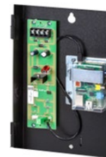
Typical mounting set-up of a SNU module
