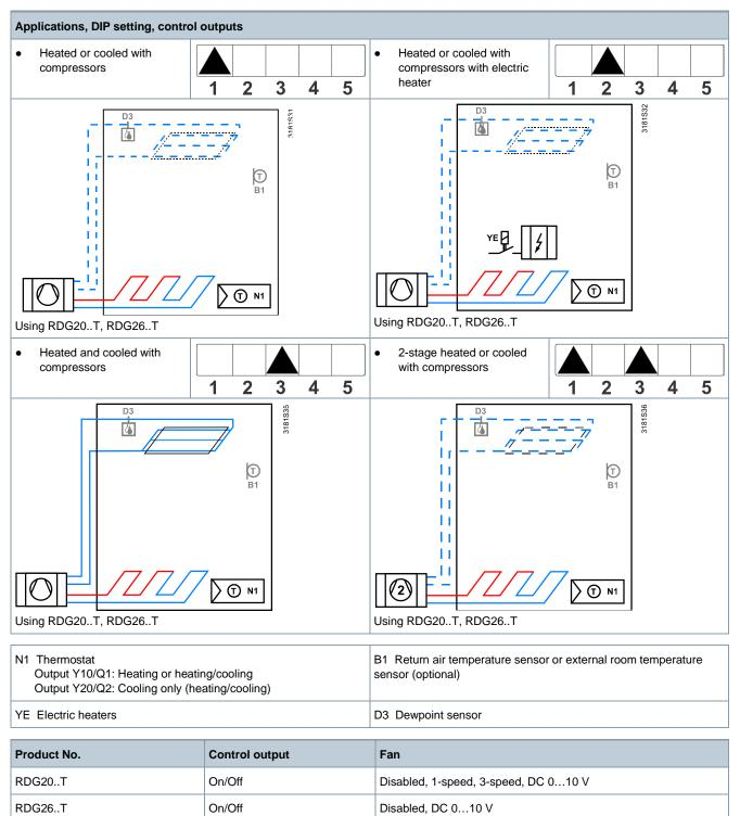
For fan coil units, universal applications and compressors in DX-type equipment applications
