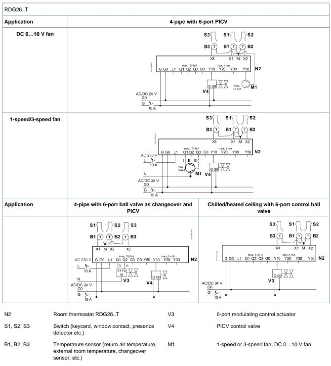
**Note**: In application "4-pipe with 6-port ball valve as changeover and PICV", Y50 can be connected with a DC 0...10 V fan.
