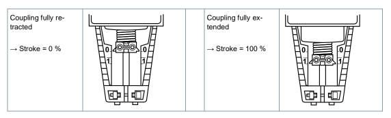
The hand crank must be rotated counter-clockwise to the end stop, i.e. until the red indicator marked "MAN" is no longer visible. This closes the Siemens valves of the series VVF.., VVG.., VXF.. and VXG.. (stroke = 0 %).
